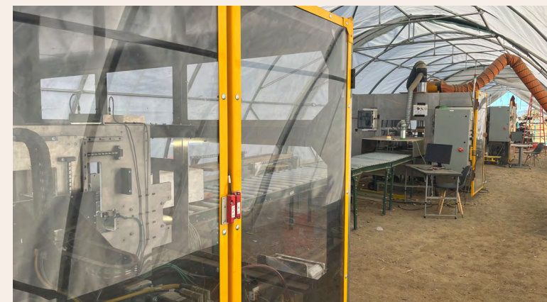
Urban Machine's processing line is almost 120 feet long and 30 feet wide. Four different robot arms move around each other in order to pick the lumber free of metal nails and other fasteners.
